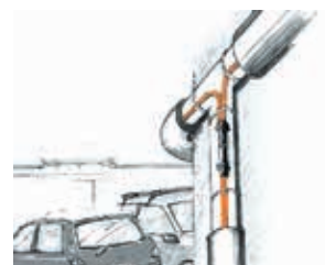
Frost protection of oil pipes
