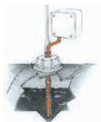
Frost protection of oil pipes
