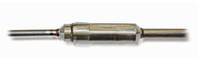
Laser welded connexion
