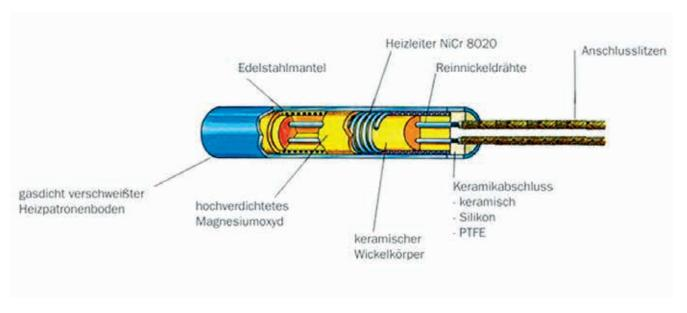
The small distance between the heating conductor and the sheath ensures both excellent heat transfer and very good control behaviour. Due to this special design, high power can be accommodated in a very small space.
